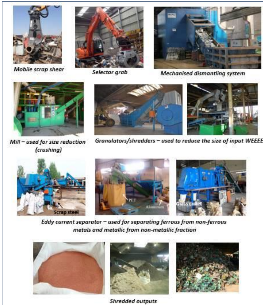
Figure 10: Type of equipment used in ICT & household equipment pre-processing
