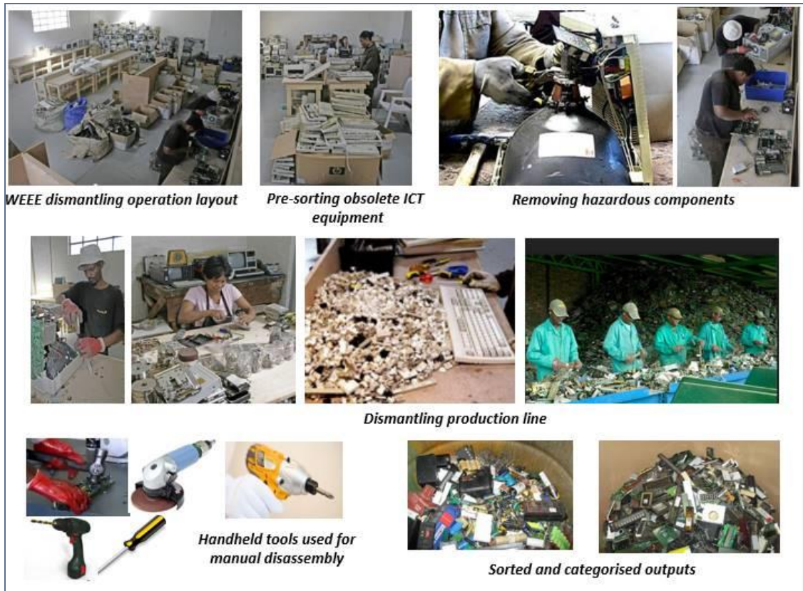
Figure 9: Manual dismantling production process in South Africa
