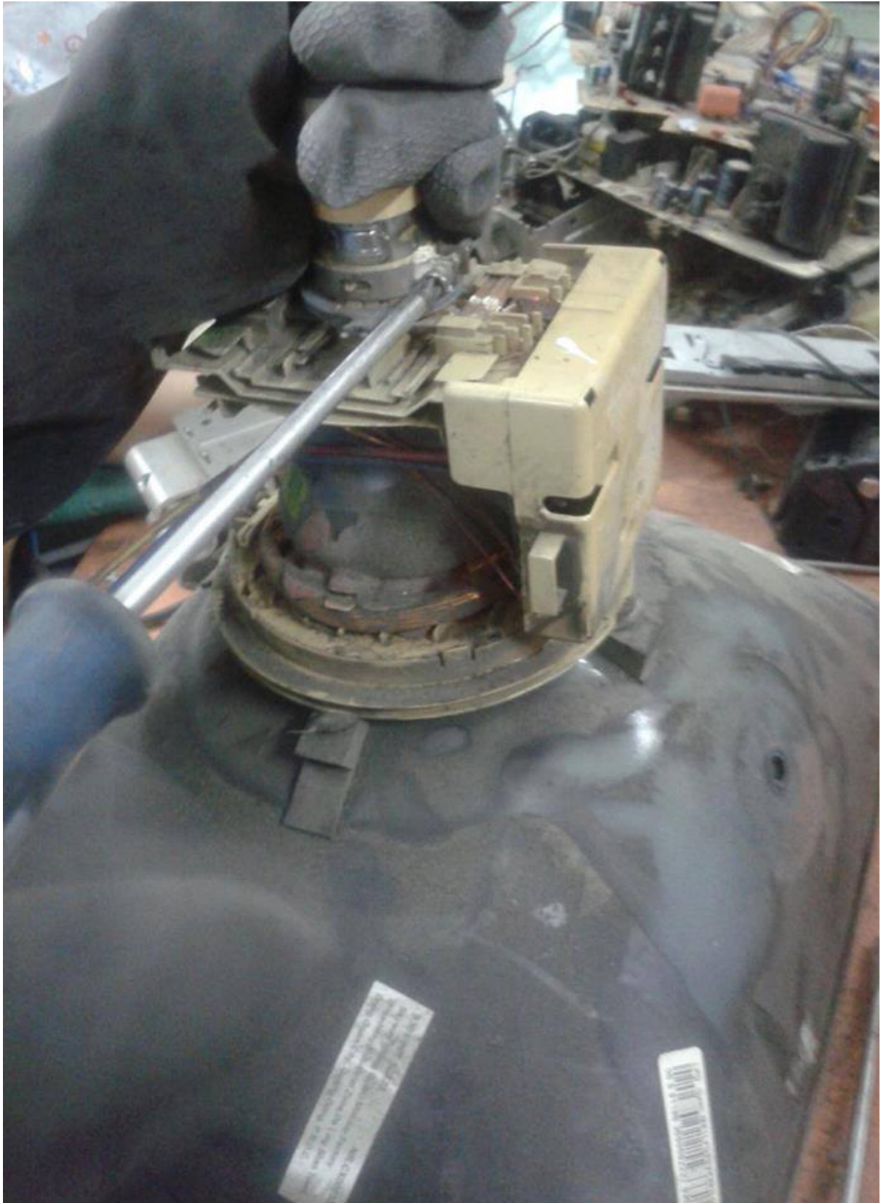
Dismantling the CRT Components including PCB
