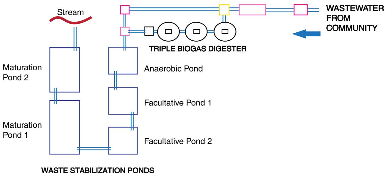
FIGURE 7. TREATMENT PROCESSES OF THE WSP SYSTEM AT CHIRAPATRE, KUMASI, GHANA (SOURCE: MODIFIED FROM YEBOAH-AGYEPONG ET AL. 2019).
