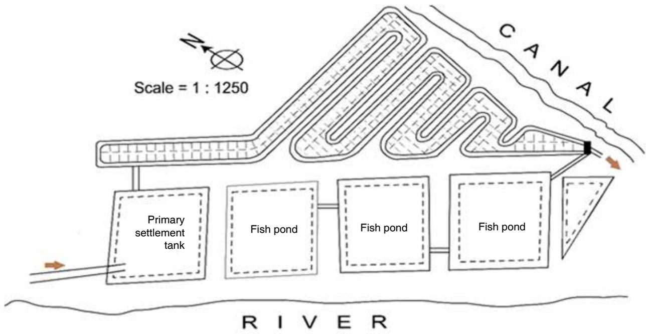
**FIGURE 11.** LAYOUT OF THE WASTEWATER TREATMENT SYSTEMS AND FISH-FARMING COMPONENTS AT AGRIQUATICS. (SOURCE: DRECHSEL ET AL. 2018, AFTER IQBAL 1999).
