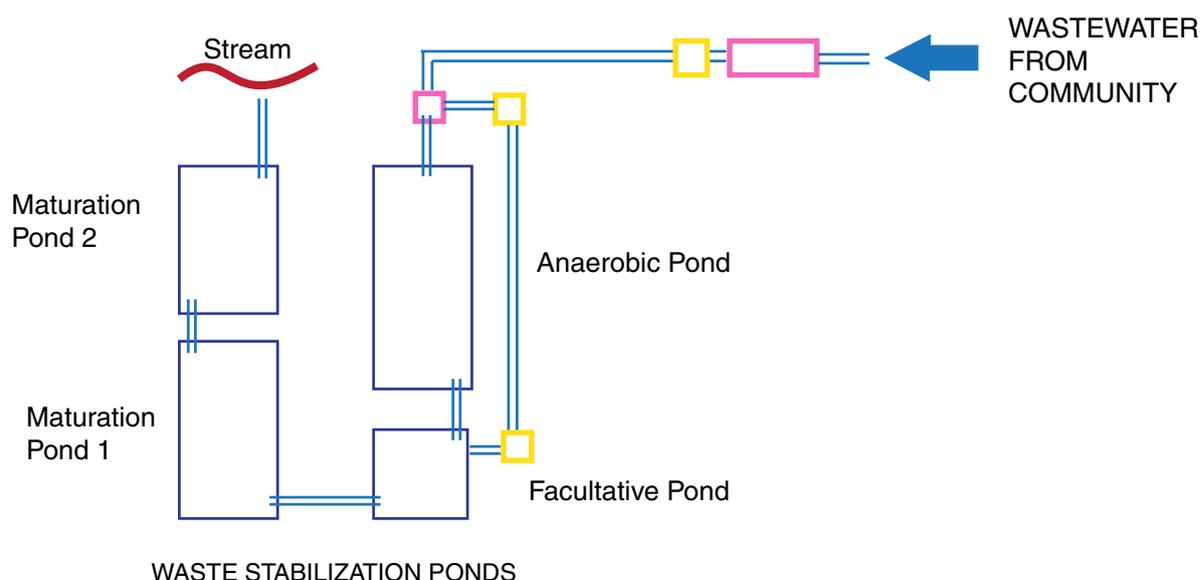
**FIGURE 3.** TREATMENT PROCESSES OF THE WSP SYSTEM AT AHINSAN, KUMASI, GHANA.
