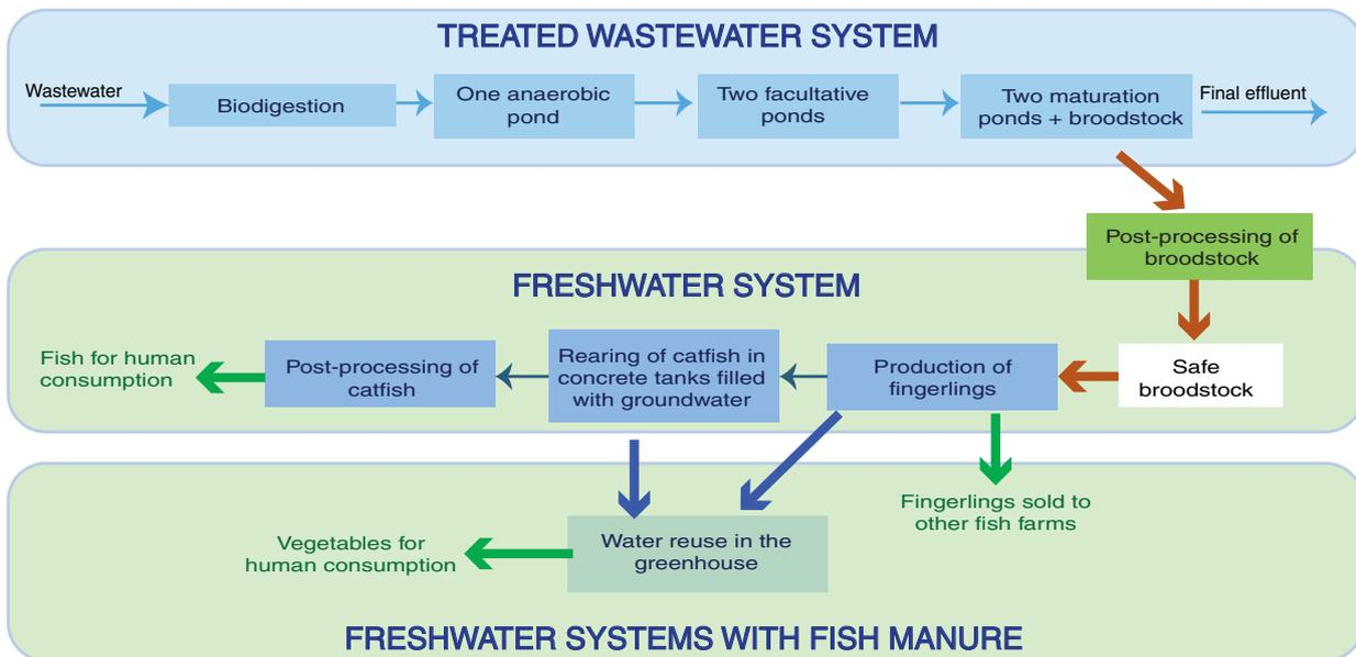
FIGURE 6. THE TAC PRODUCTION PROCESS AND VALUE CHAIN AS OF 2020.
