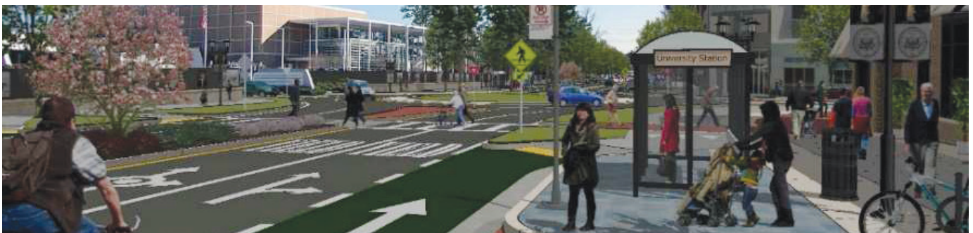
FIGURE 1.7: An example of a complete street An artist's impression of a complete street, allowing for the safe, simultaneous use of the street by pedestrians, motorists and cyclists. Also notice the combination of hard and soft landscaping elements, the use of colour in paving choices, clear signage and road markings, and attractive and functional street furniture. Source: blog.aarp.org
