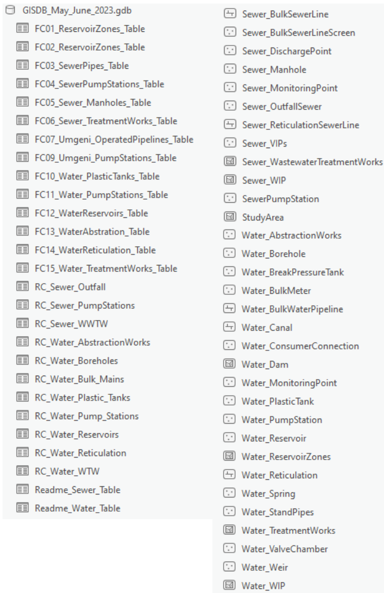
Diagram 1: The custom designed Geodatabase, showing the layout of the feature classes and tables within the geodatabase.
