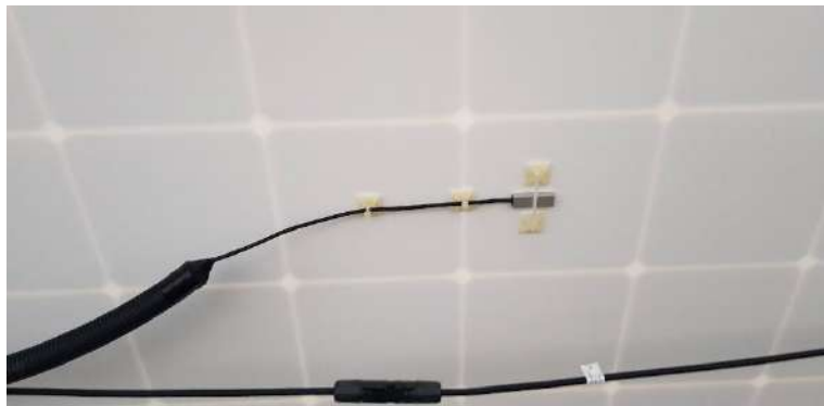
Figure 35: Typical back of module temperature sensor
