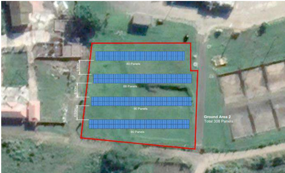
Figure 28: Area 2 - Ground-mounted bifacial tracking solar system
