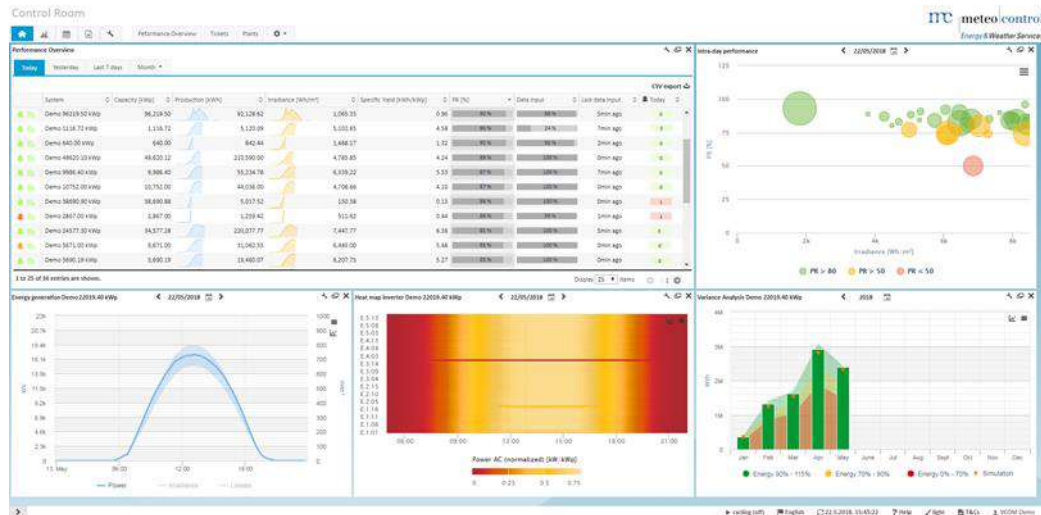
Figure 32: Typical dashboard of PV facility monitoring system
