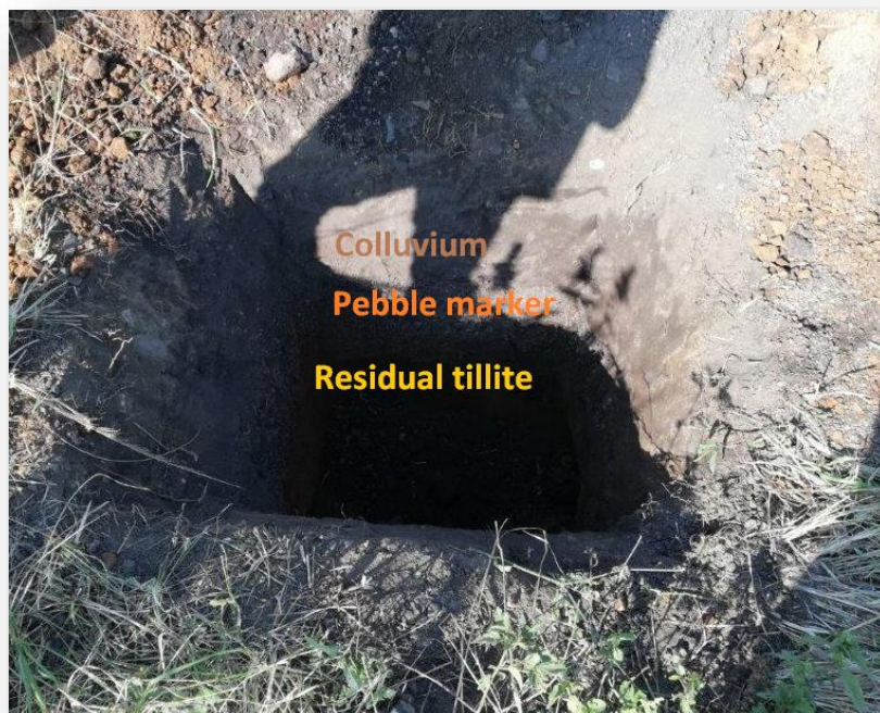
Figure 6: Typical test pit showing subsoil profile.
