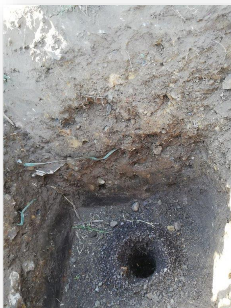
Figure 5: Fill retrieved from a test pit.
